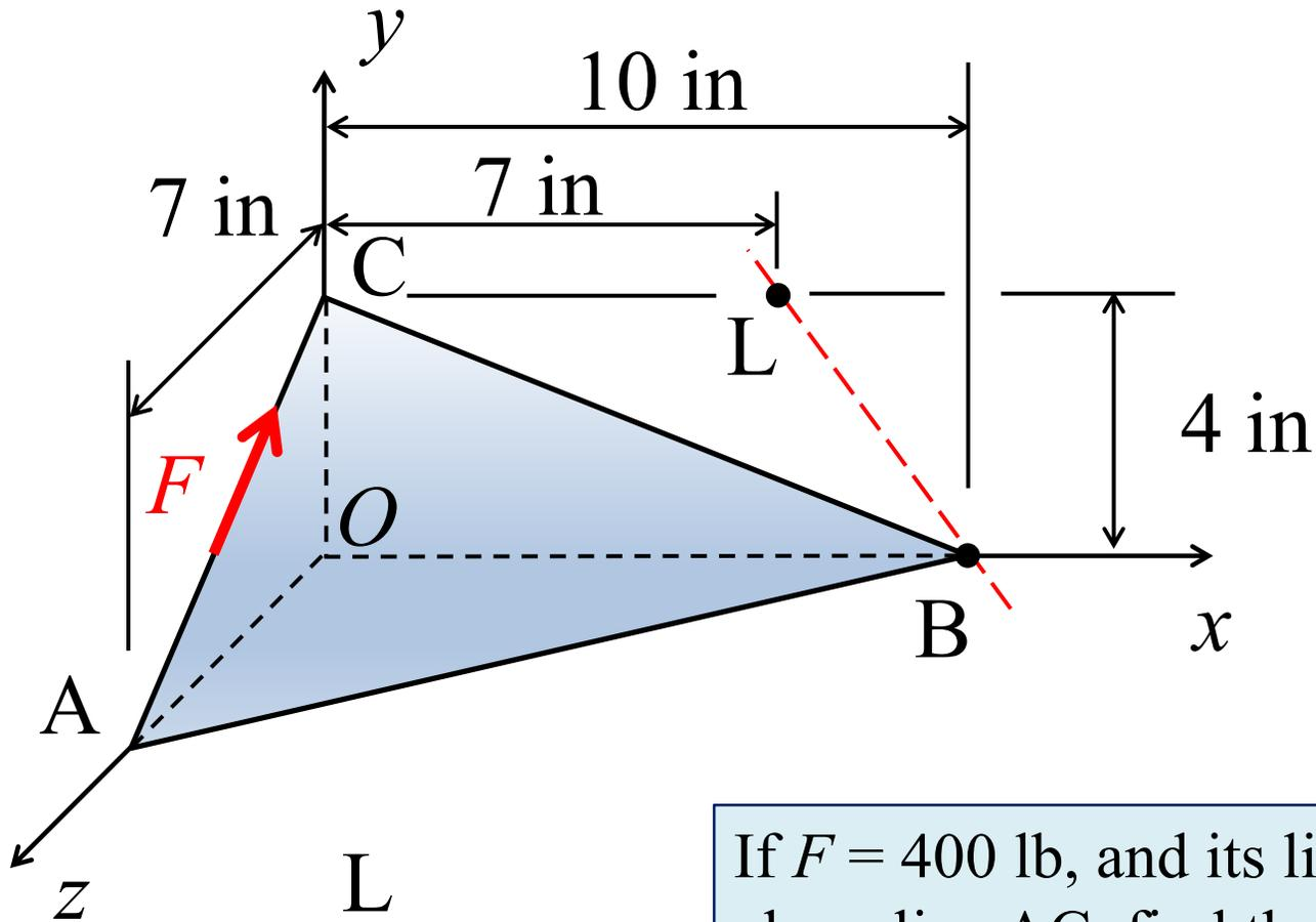
If  $F = 400$  lb, and its line-of-action lies along line  $AC$ , find the moment of the force about the axis defined by line  $BL$  that lies in the  $xy$  plane.
